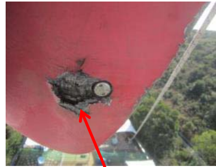
Damage of Blade tips around Lightning Receptor
